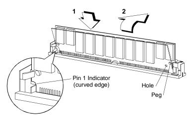
**CAUTION:** A SIMM fits only in one direction. If you slip in a SIMM but it does not appear to completely fit, you may have inserted it the wrong way.
